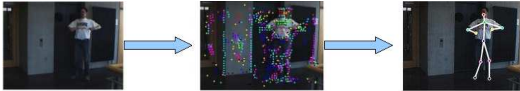
Figure 2: Left: Input test image. Middle: Possible candidates (dots) for different body parts detected by local classifiers. Right: Detected human with pose found by using graphical inference.
